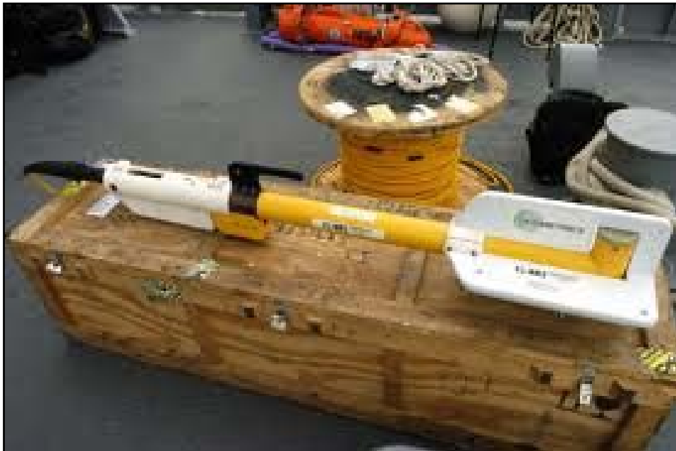
Plate 3. Geometrics 882 Marine Magnetometer
